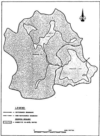
Figure III 1.6 Bedrock geology and basin designation of the Crosson Lake watershed
