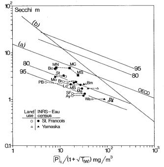
Figure II 10. Secchi transparency in relation to flushing corrected inflow total phosphorus concentration
