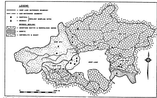
Figure III 1.10 Bedrock-geology, sampling sites and besin designation of the Harp Lake watershed
