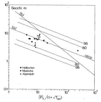
Figure II 17. Secchi transparency in relation to flushing corrected inflow total phosphorus concentration
