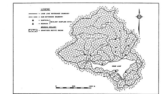
Figure III 1.5 Bedrock geology, sampling sites and basin designation of the Chub Lake watershed
